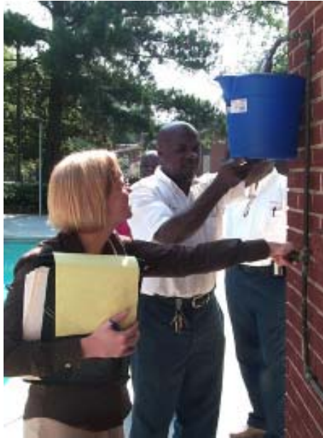
P 2 AD's Judy Adler and Amara Conteh of the Lenox Woods Apartments test the flow rate from a spigot.
